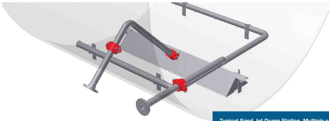
Typical Sand Jet Dump Station. Multiple sand jet / dump stations provide for calibrated solids removals sequencing.
