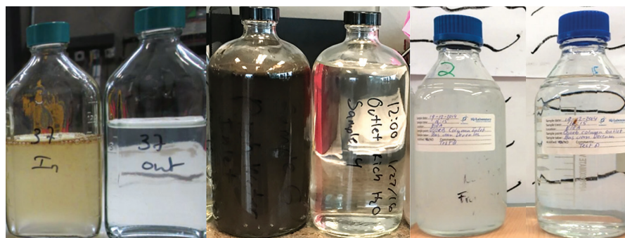
Dispersed oil removal during pilot scale polymer testing. (ProSep 2017)
