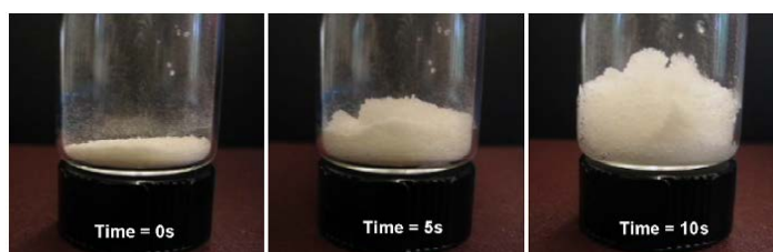
Figure 1.B – Images of Osorb expanding as it adsorbs organics. (Edmiston, 2009)
